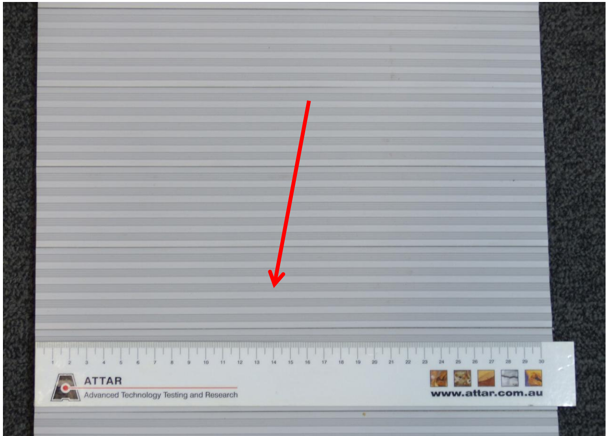
Figure 1: Roberts Wide Ribbed stair insert 50mm 15-0007-03 Arrow indicates direction of testing
